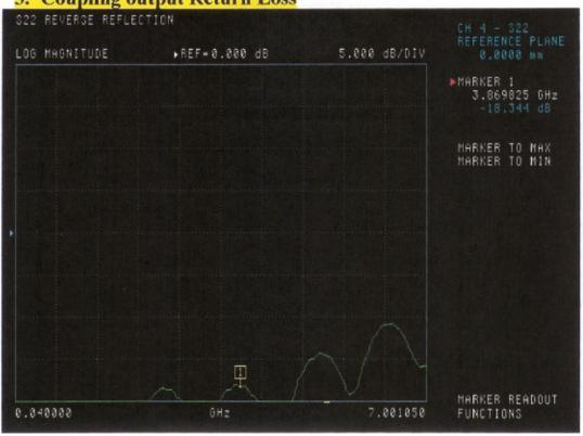
4. Residual Return Loss on probed line
